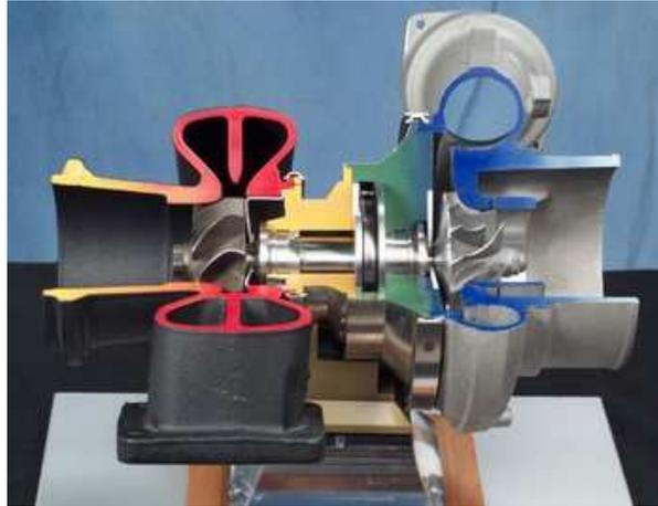
A turbosupercharger is a device used in internal-combustion piston-engines to increase the power output of the engine by increasing the mass of oxygen and fuel entering the cylinders. A key advantage of turbosuperchargers in aircraft is that they offer a considerable increase in engine power with little weight increase.
